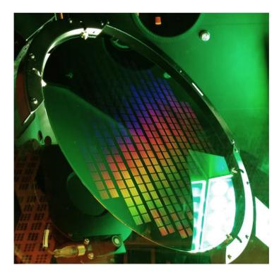
First exposures after upgrade to fully programmable blanker
